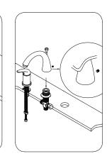
Unscrew the Allen screw in back of the spout. Pull apart the spout from its connector (do not unscrew). Separate the spout flange from the spout. Place o-ring underneath the spout flange and place the flange over the center hole between the handle and hand shower.
