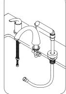
Unscrew the locknut and take off metal and rubber washers.
